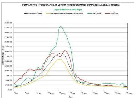
The hydrological situation in the Niger basin during the month of February was characterized by a continued decline in flows across the entire basin except the Lower Niger sub- basin. The Selingué dam in Mali has begun gradual release to support downstream flow.
